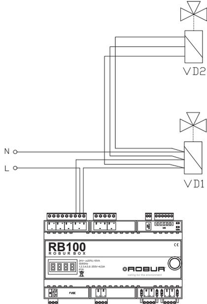
VD1 system delivery pipes 3-way motorised valve
