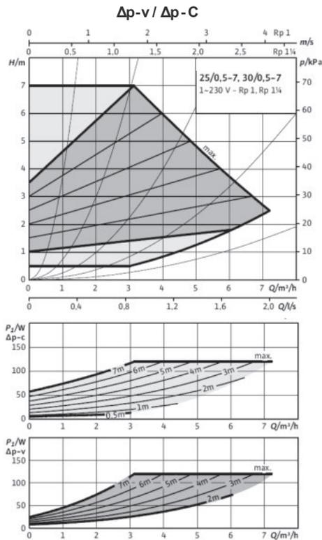
**Figure 2.2** Oversized pressure head circulating pump characteristic curves
