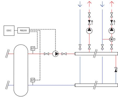
ST Temperature probes on secondary circuit
