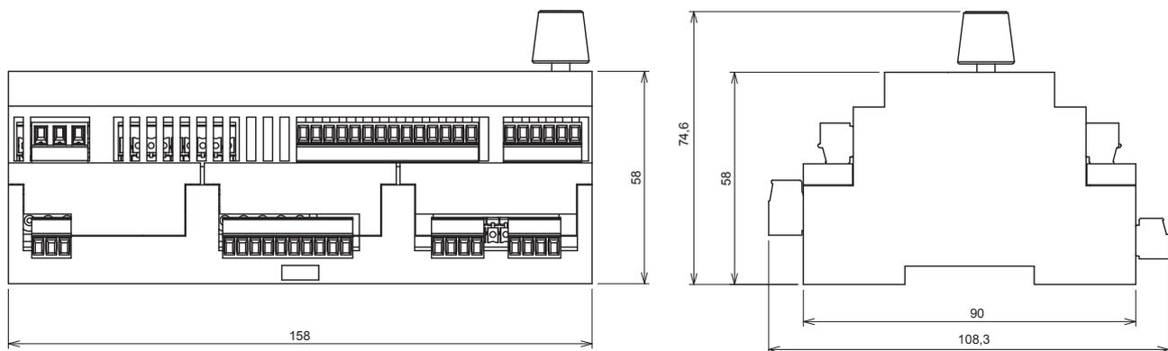
The RB200 device has protection rating IP20, and must be installed in premises with ambient air temperature between 0°C and 50°C.
