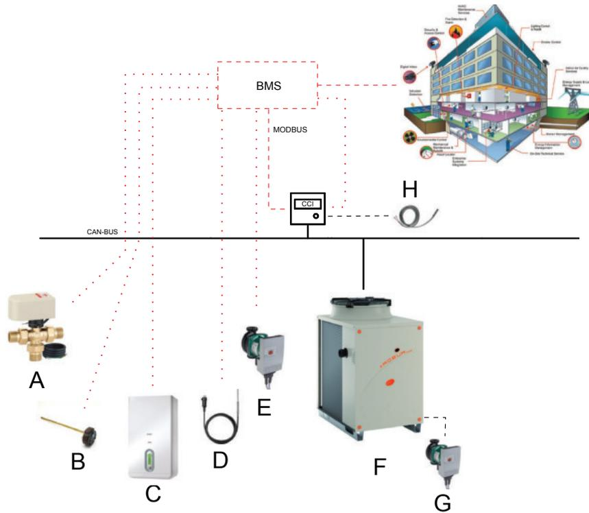
In solid line the CAN-BUS connection connecting Robur control devices to the units
