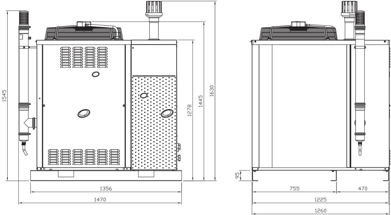
**Figure 2.2** Dimensions (Silenced ventilation) - Front and side view (dimensions in mm)
