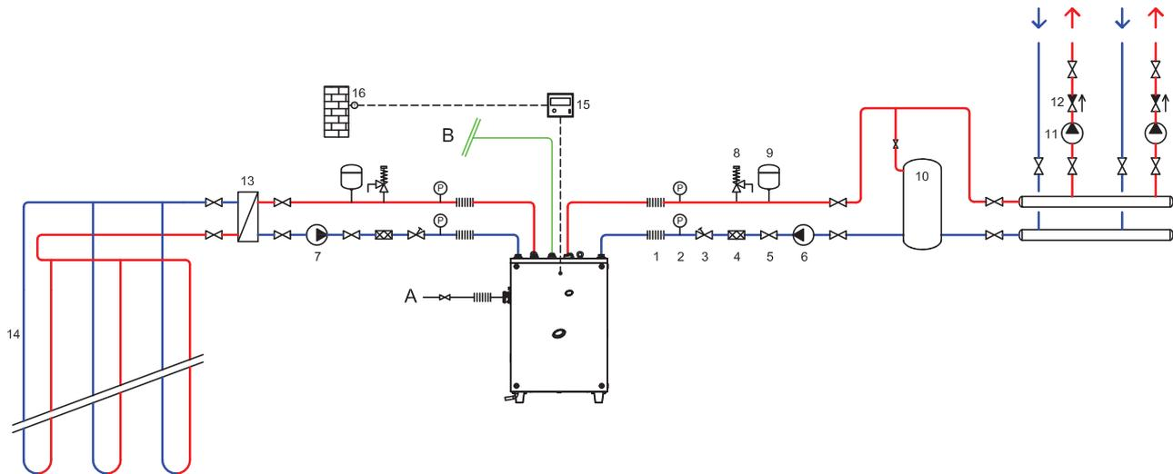
The flow regulator valve must only be used when the primary circuit circulation pump is constant flow type
