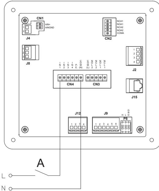
A Enable turning on request from external controller
