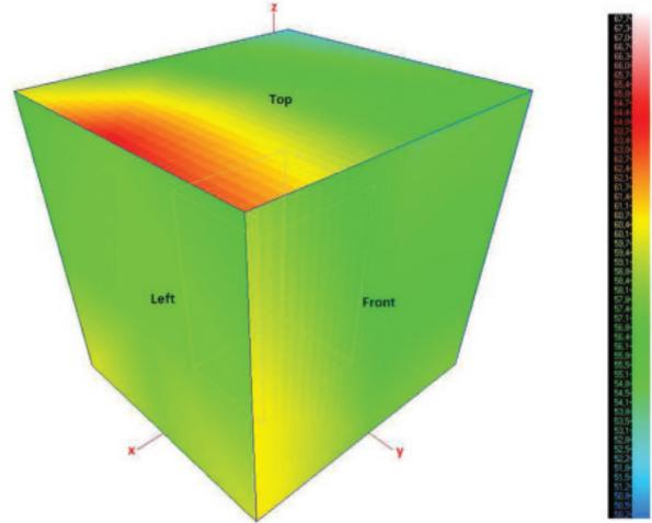
Sound intensity measured on unit GAHP GS/WS surface, front, top and left side view
