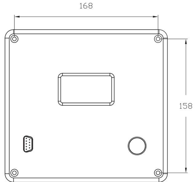
The CCI Panel has protection rating IP20, and must be installed in premises with ambient air temperature between 0°C and 50°C, away from direct sunlight exposure.
