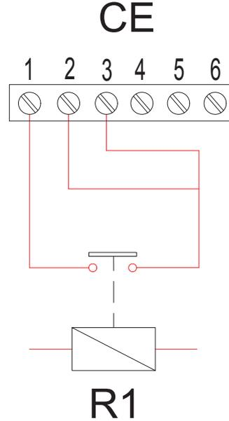
Details of CE connector (see Figure 2.2 p. 4)
