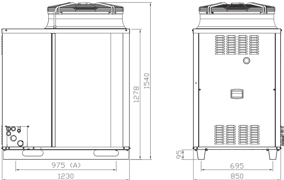
A Position of holes for fixing of anti-vibration joints
