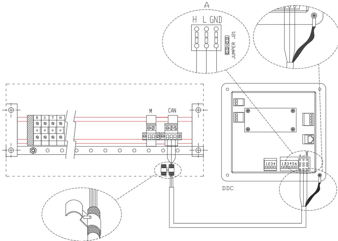
CAN 3-pole connector for CAN-BUS network connection
