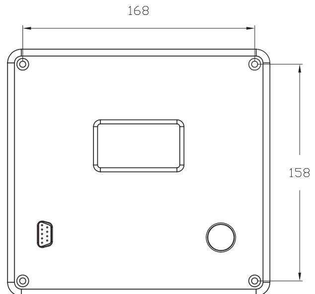
The DDC Panel has IP20 degree of protection, and must be installed in premises with ambient air temperature between 0°C and 50°C, away from direct sunlight exposure.
