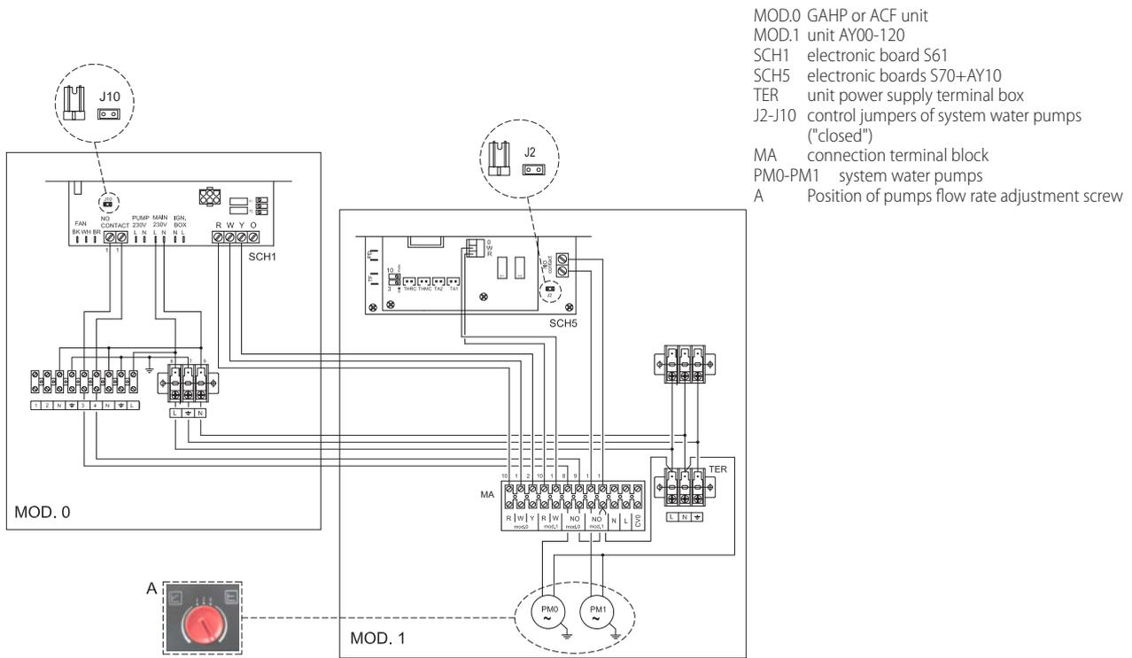
Figure 3.6 CAN connection between AY10 board and S61 (pre-wired in the factory)
