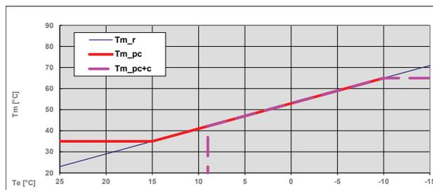
Tm\_r Delivery temperature required by the system (linear weather curve)
