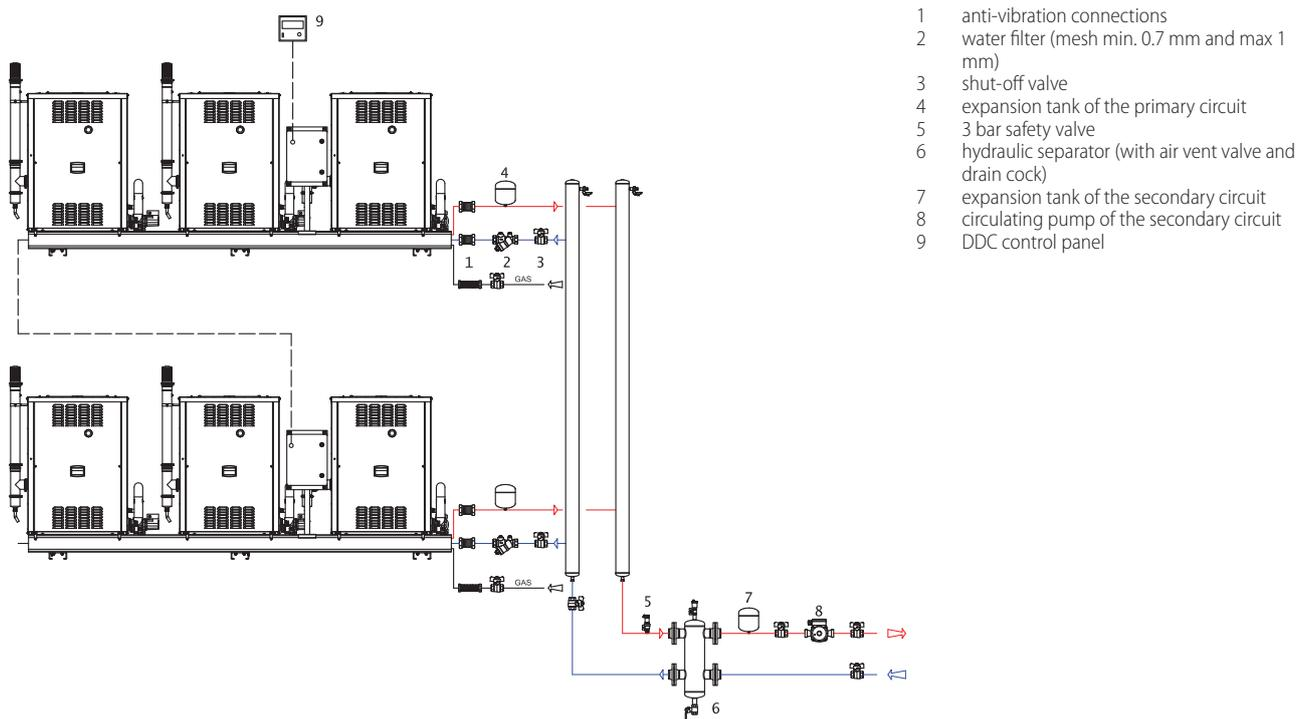
Figure 1.6 Example of hydraulic system diagram for connection of n. 1 RTCR version without circulating pumps
