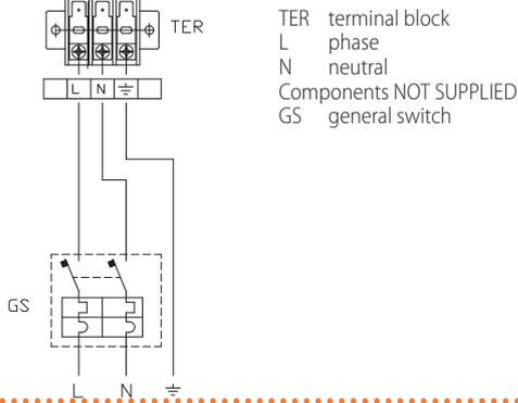
The switches must also provide disconnecter capability, with min contact opening 4 mm.
