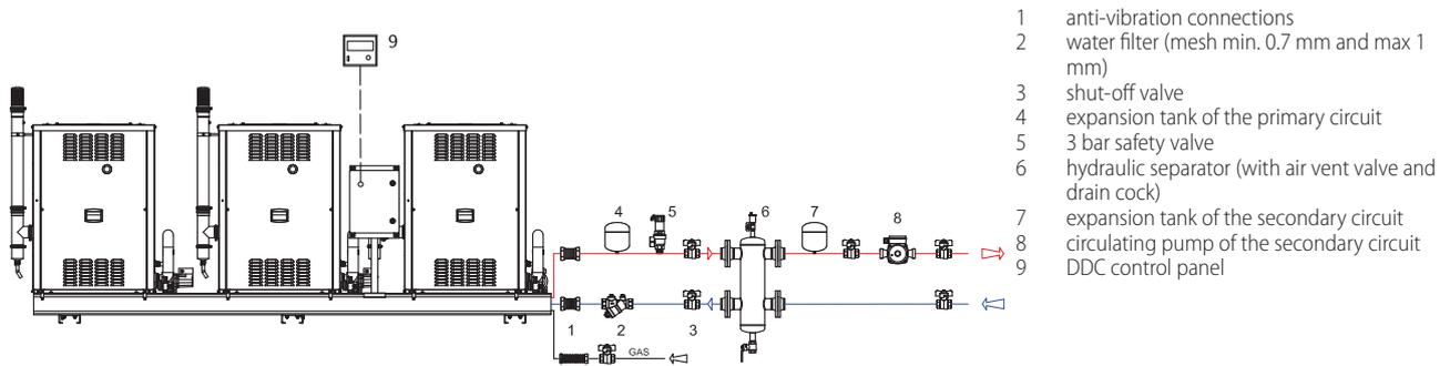
**Figure 1.5** Example of hydraulic system diagram for connection of n. 2 RTR, version with circulating pumps
