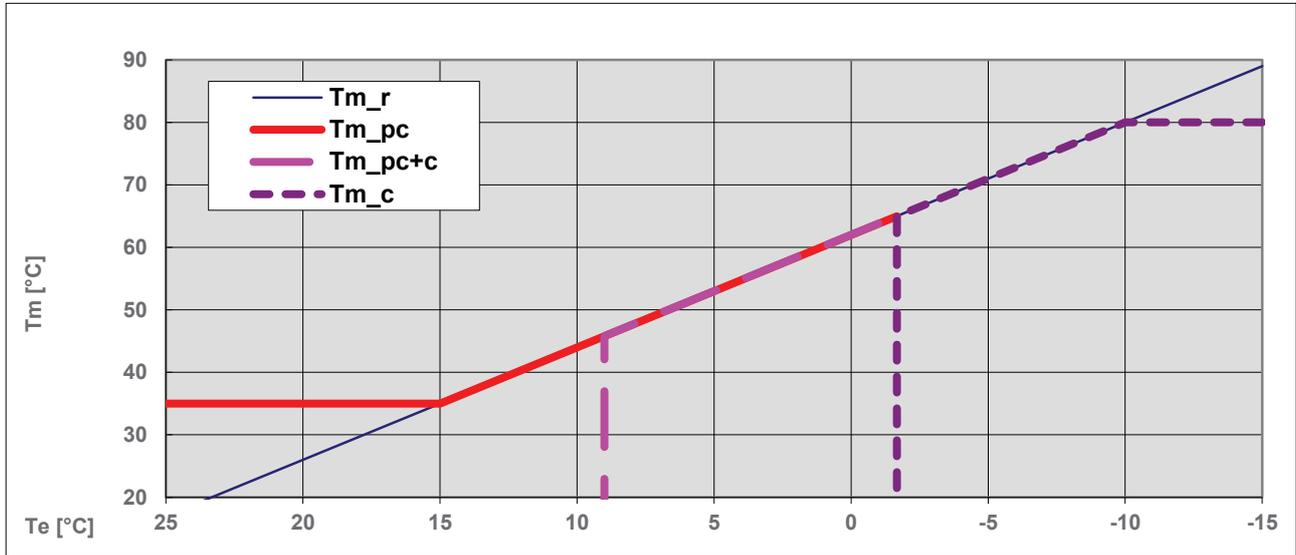
Tm\_r Delivery temperature required by the system (linear weather curve)
