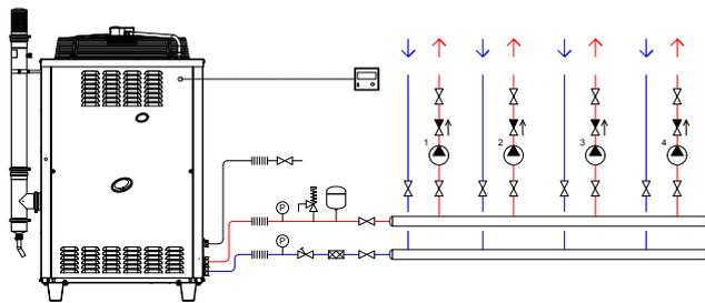
In general these systems characterized by strong imbalances in the flow rates are unlikely to work under the design conditions and therefore to ensure efficiency and comfort.
