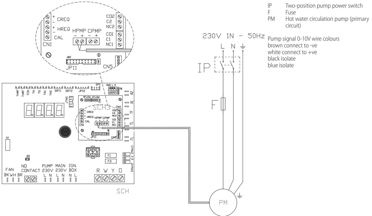
**Figure 3.10** Wiring diagram for hooking up the Wilo Stratos Para variable rate pump powered by the unit
