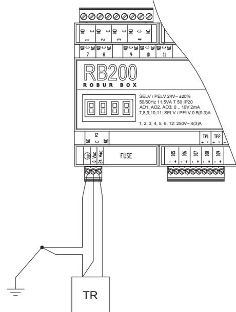
TR Safety transformer 230 Vac/24 Vac min 12 VA (not supplied)
