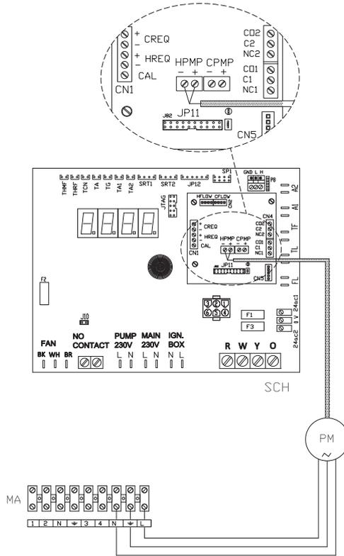
PM Hot water circulation pump (primary circuit)
