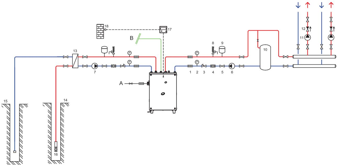
The flow regulator valve must only be used when the primary circuit circulation pump is constant flow type
