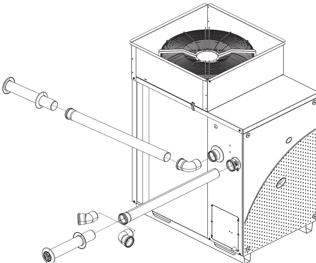
Figure 3.2 Type C53 roof flue gas exhaust
