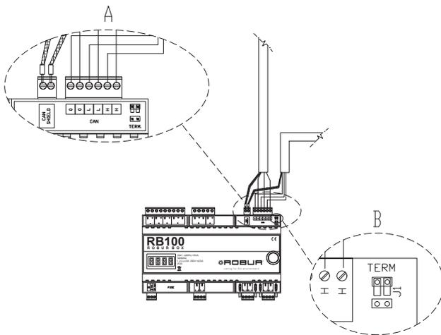
A CAN-BUS screen connection detail
