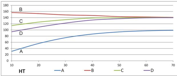
In abscissa the power percentage with GAHP compared to the design power (both calculated at conditions A2W55)
