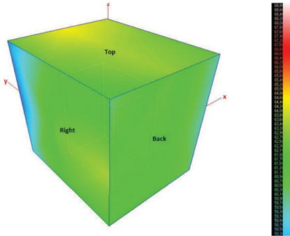
Sound intensity measured on unit GAHP A HT S1 surface, rear, top and right side view
