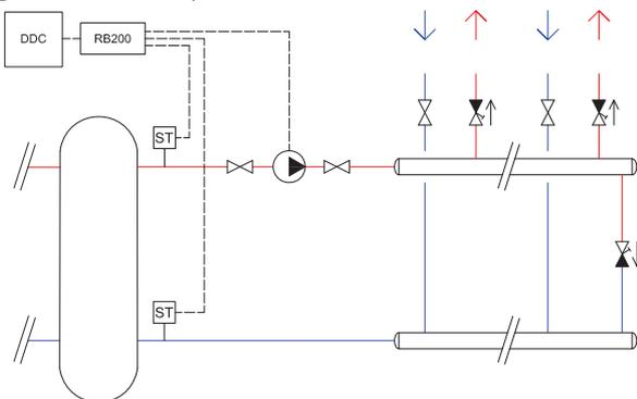
ST Temperature probes on secondary circuit
