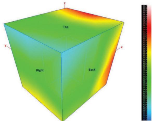
Sound intensity measured on unit GAHP GS/WS surface, rear, top and right side view
