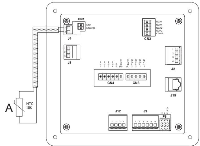
A Heating manifold delivery or return probe
