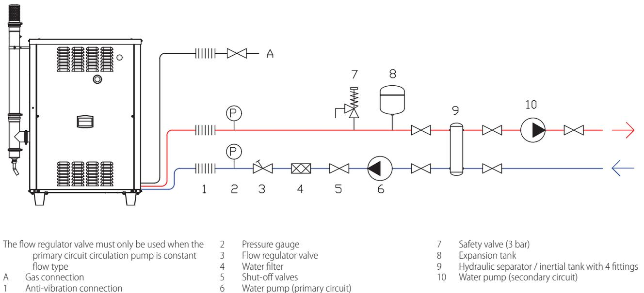
Figure 1.2 p. 2 shows an example of plumbing diagram for an individual GAHP GS HT unit.
