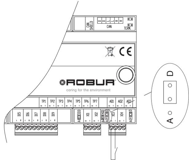
**Diverter valve outputs**
