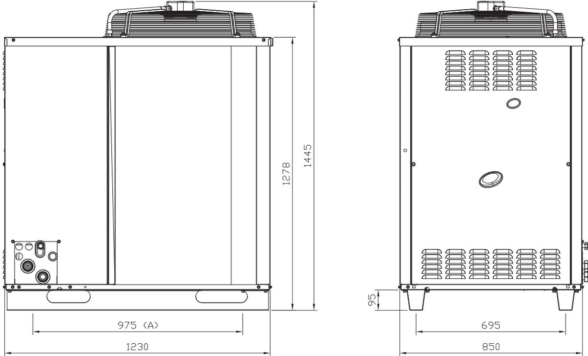
A Position of holes for fixing of anti-vibration joints
