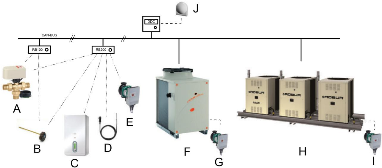
In solid line the CAN-BUS connection connecting control devices Robur
