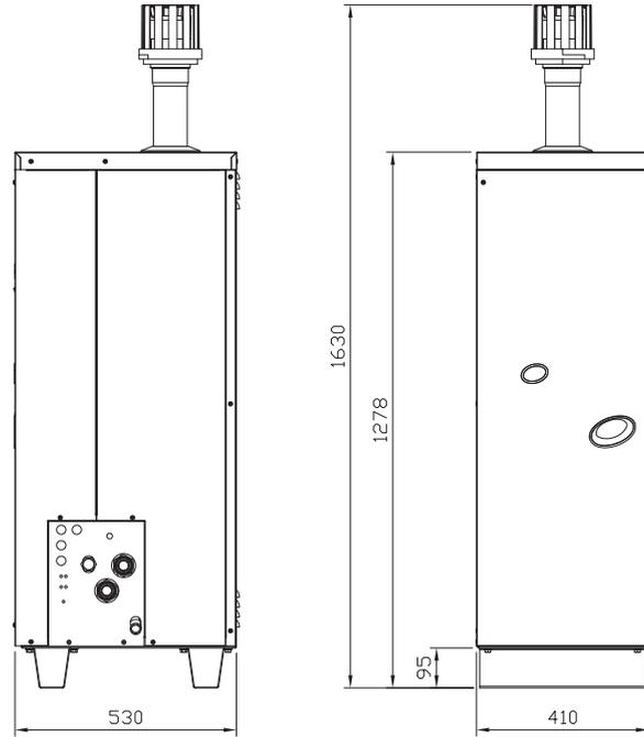
**Figure 2.2** Service plate - Hydraulic/gas unions detail
