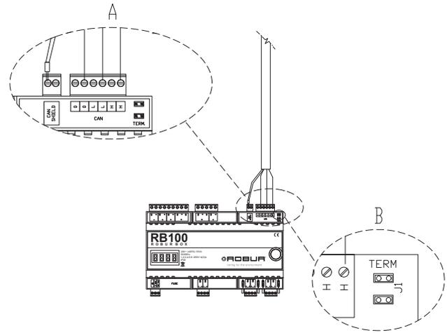
A CAN-BUS screen connection detail
