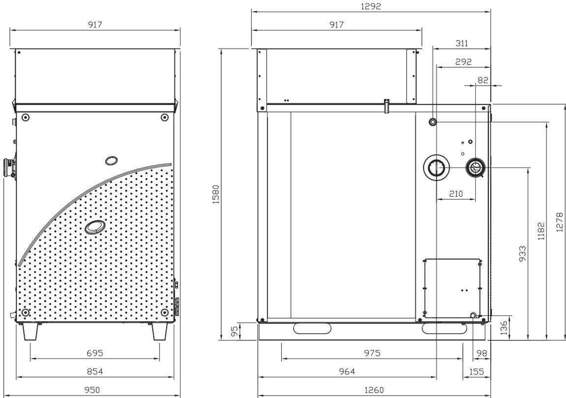
**Figure 2.2** Service plate - Hydraulic/gas unions detail
