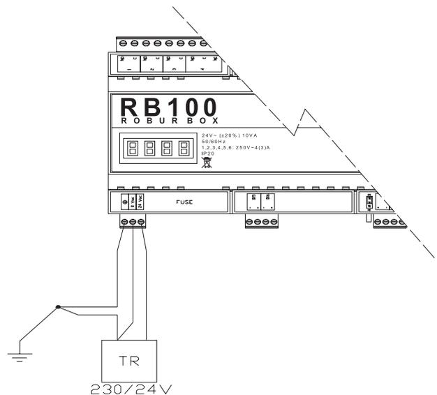
TR Safety transformer 230 Vac/24 Vac min 10 VA (not supplied)
