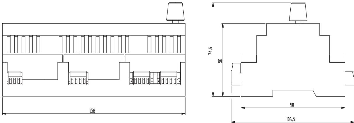
The RB100 device has protection rating IP20, and must be installed in premises with ambient air temperature between 0°C and 50°C.
