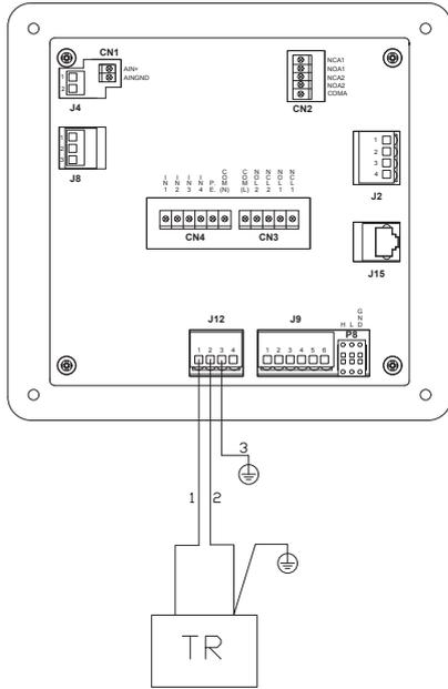
J12 24 Vac electrical power supply - 4 pole connector
