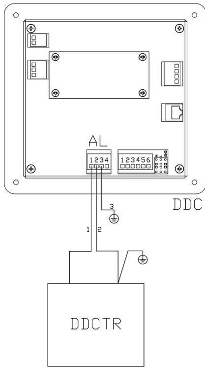
AL = 24 Vac electrical power supply - 4 pole connector
