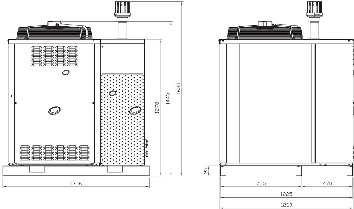
**Figure 2.2** Dimensions (Silenced ventilation) - Front and side view (dimensions in mm)
