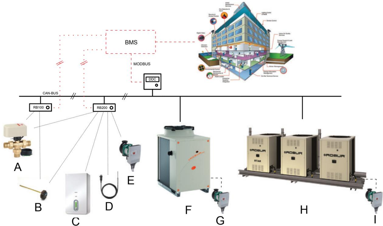
In solid line the CAN-BUS connection connecting control devices Robur
