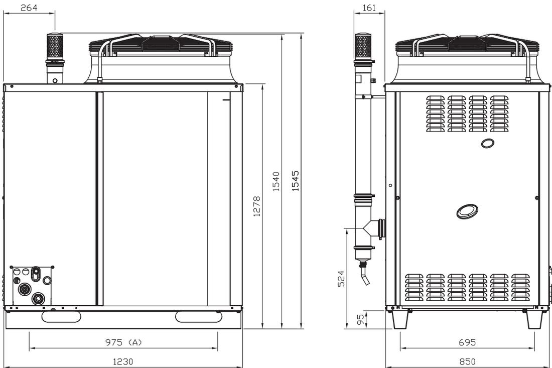
A Position of holes for fixing of anti-vibration joints
