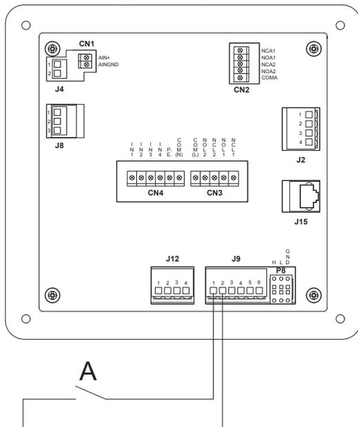
A Auxiliary generator turning on signal from external controller
