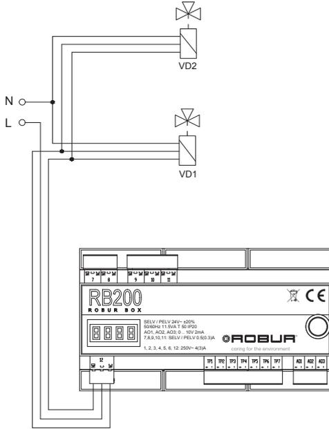
VD1 system delivery pipes 3-way motorised valve
