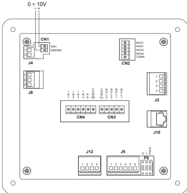
**Manifold temperature probe input**
