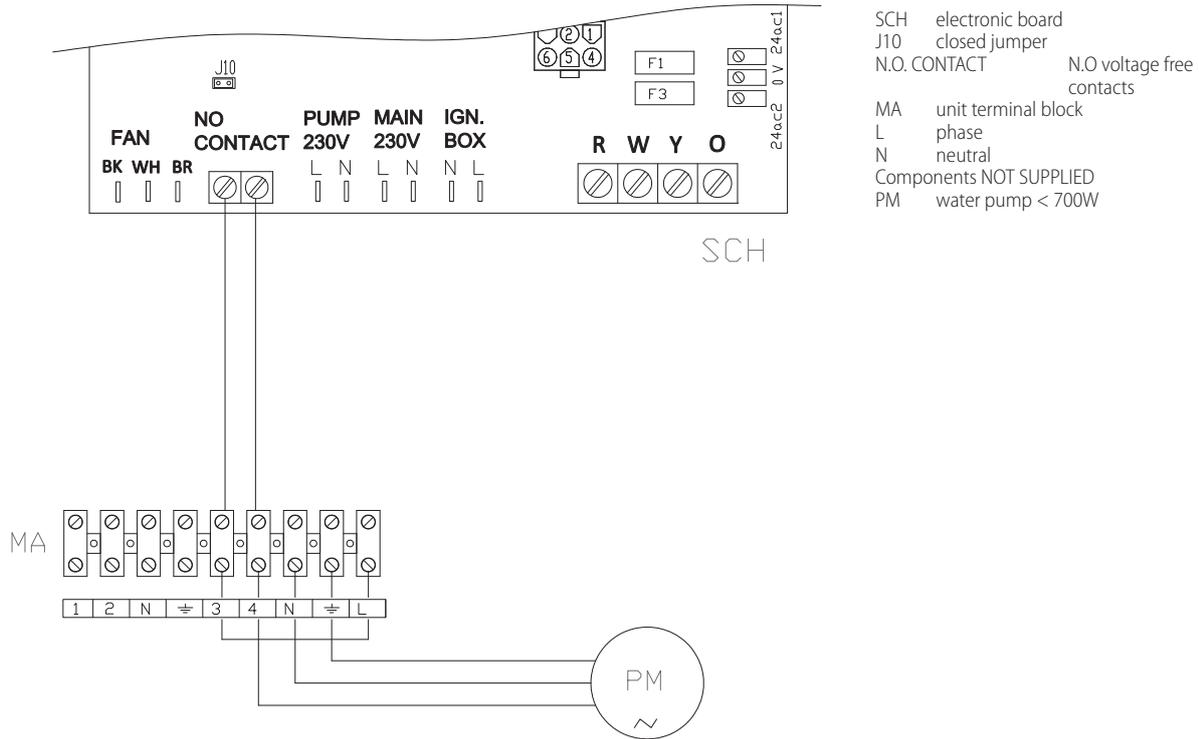
**Heat recovery exchanger circulating pump**
