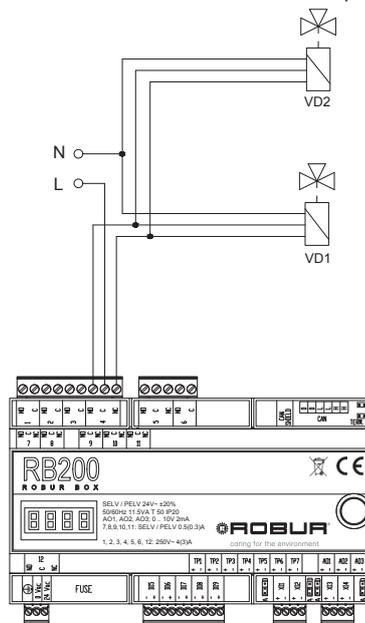
VD1 system delivery pipes 3-way motorised valve
